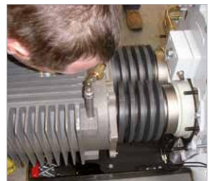
SCREWLINE pumps enable simple disassembly of the pump chamber for on-site cleaning by the customer
